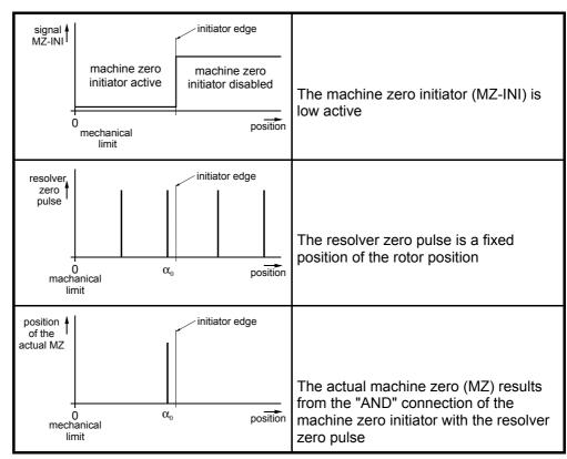
Example 1:  $\alpha_0 = 90^\circ$ ; clockwise rotating motor in direction of mechanical limitation
